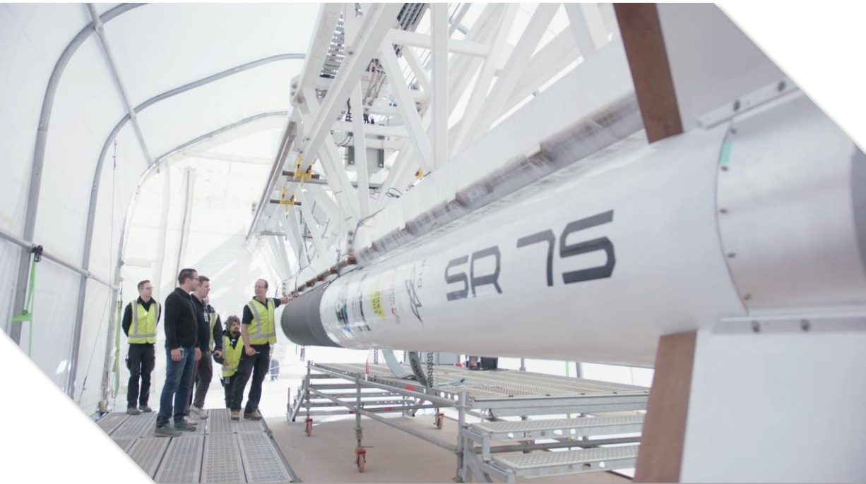
Rocket is connected to the launch rail interfaces Connection of the umbilicals
